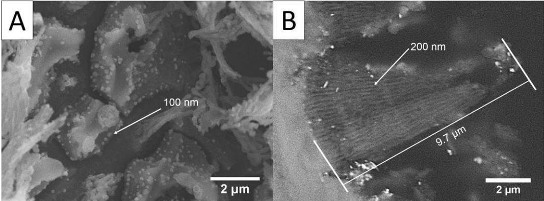
Figure 1. (A) SEM image of the oxide surface containing Ag NPs. (B) Cross-section SEM image of formed Al<sub>2</sub>O<sub>3</sub> nanotubes.
