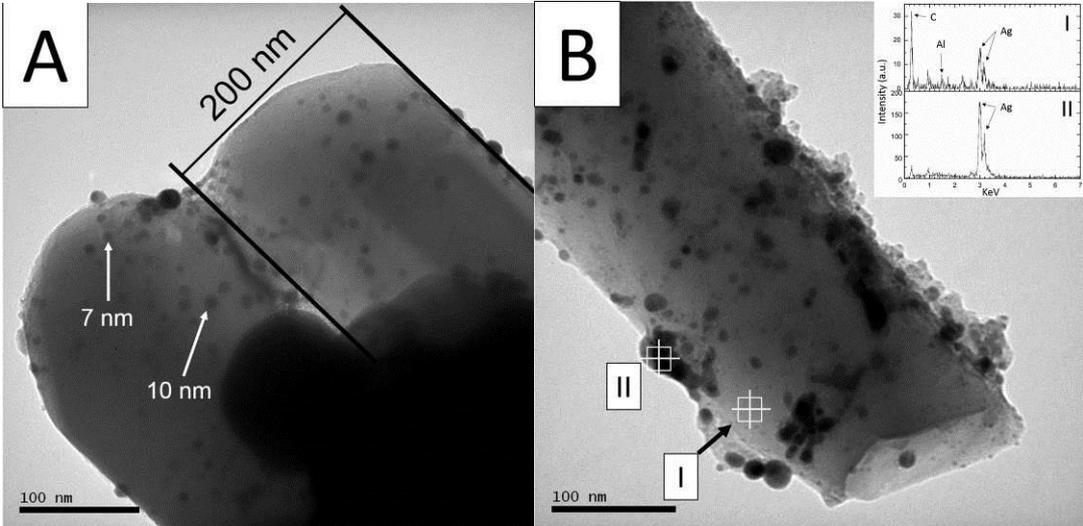
Figure 2. (A) TEM image of formed Al<sub>2</sub>O<sub>3</sub> nanotubes with embedded silver nanoparticles. (B) TEM image of nanotube showing the areas of EDS analysis. The insert shows the obtained spectra.
