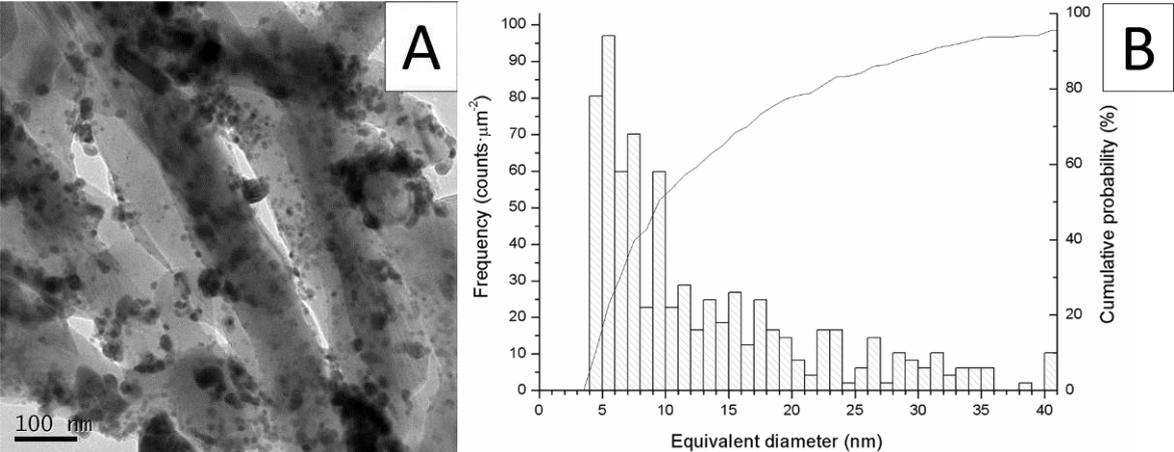
Figure 3. (A) Area selected for the distribution analysis by TEM and (B) histogram of the frequency per area versus the equivalent diameter of the silver nanoparticles and the cumulative probability.
